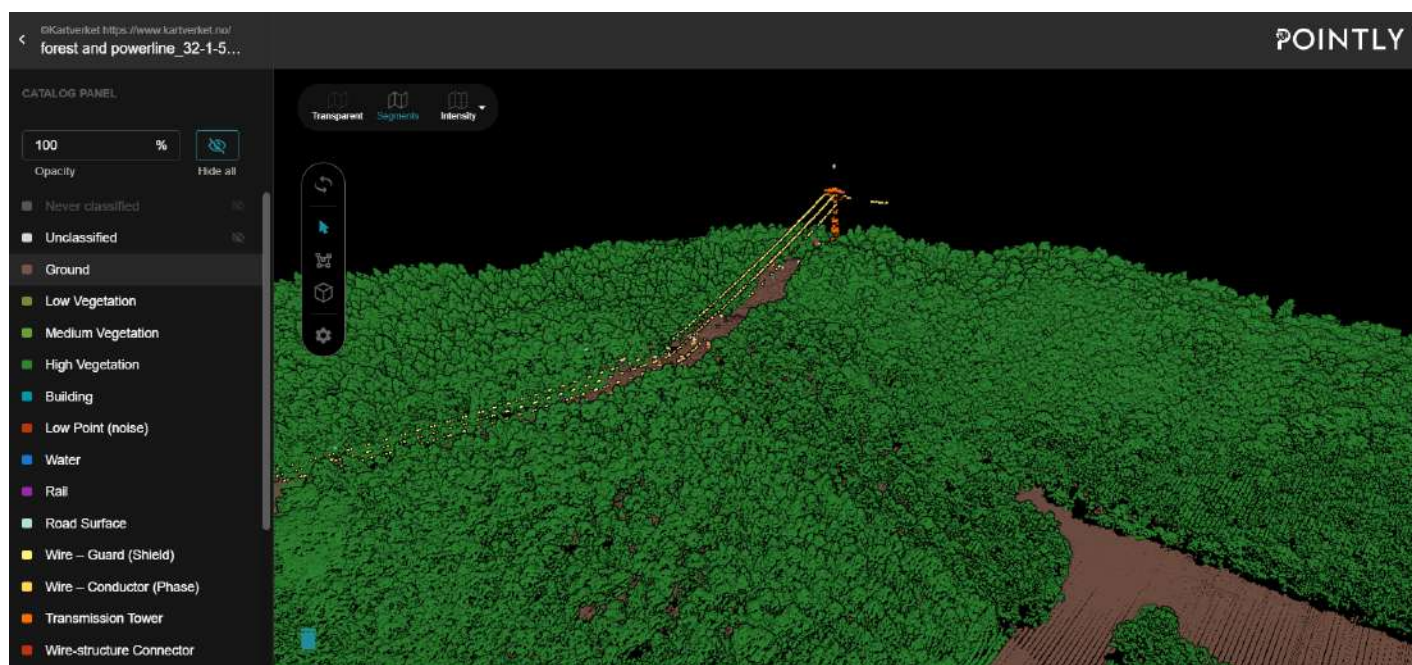
Figure 3: Classified point cloud in Pointly with vegetation, ground, powerlines (etc.).
