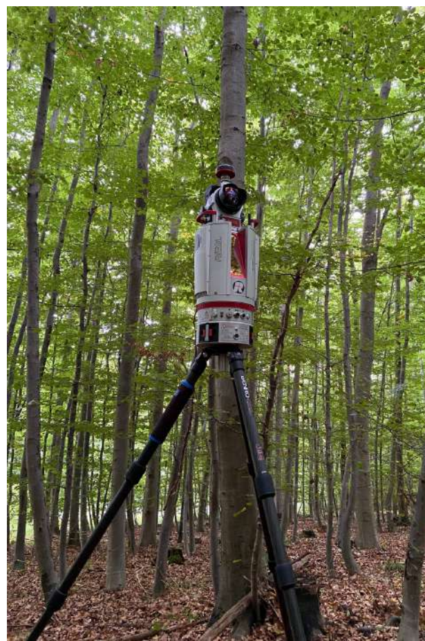
Figure 4 : A RIEGL terrestrial laser scanner at work.
