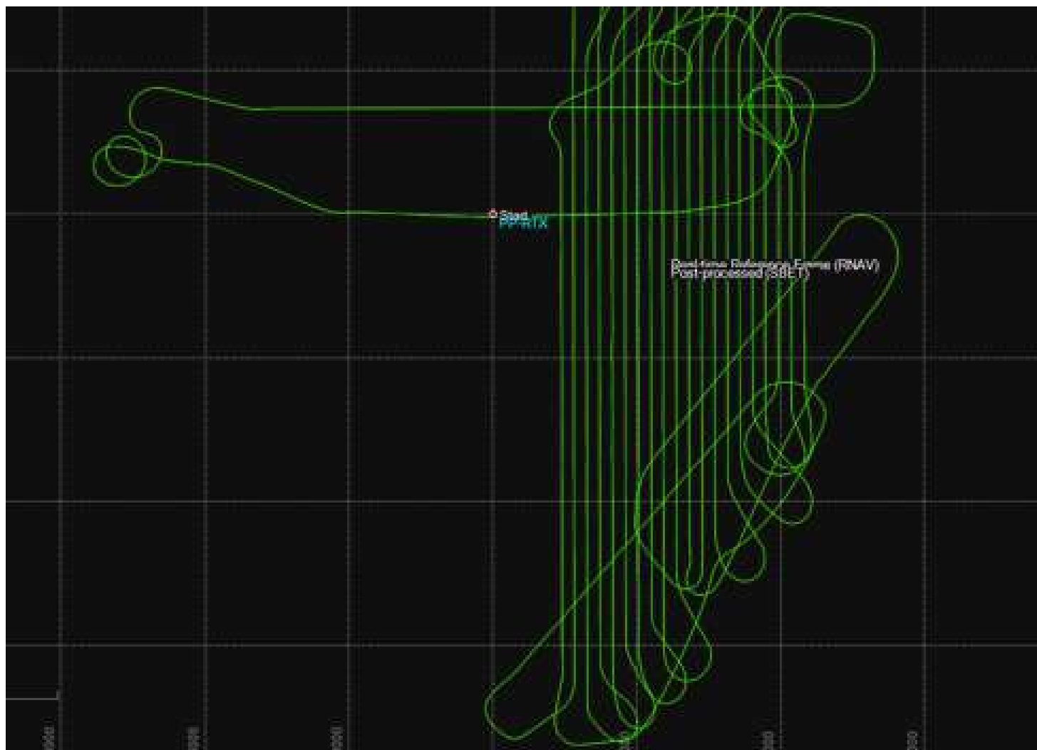
Figure 1: GNSS guidance enabled efficient flight paths for lidar surveys while RTX-PP provided precise positioning to produce accurate, high-volume terrain mapping.
