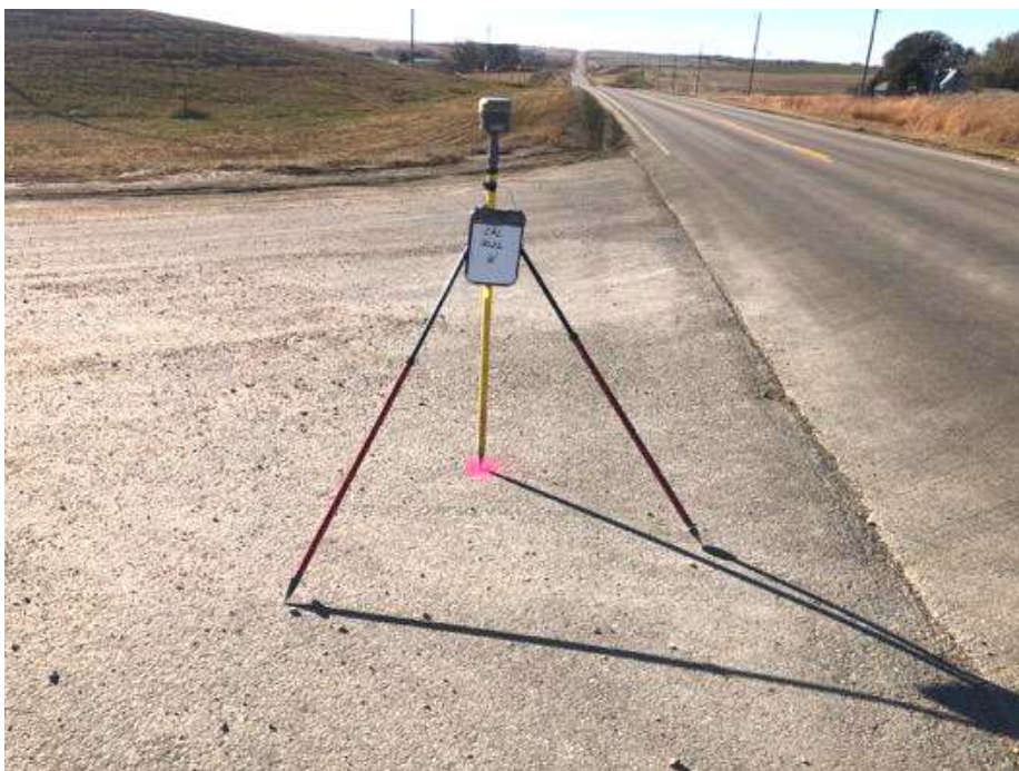
Figure 3: A Trimble R10 GNSS receiver uses CenterPoint RTX to produce precise position data. RTX enabled efficient real-time measurement without the need for base stations or cellular connections. Images are linked to the correct location.
