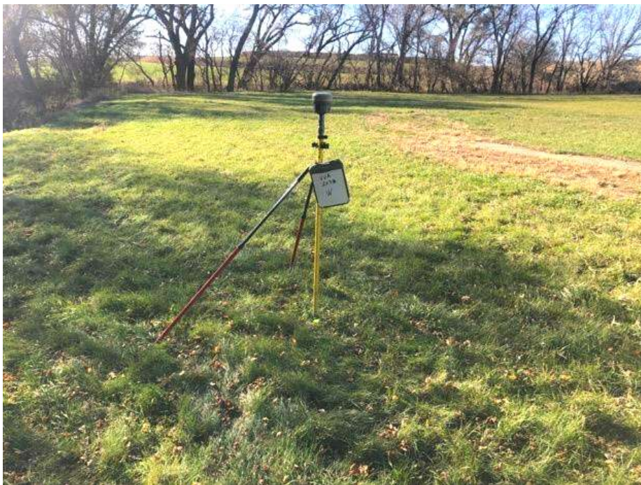
Figure 2: A GNSS receiver and RTX capture precise data while Kenna collects photos to document the site. The site identifier written on the whiteboard ensures the data and images are linked to the correct location.
