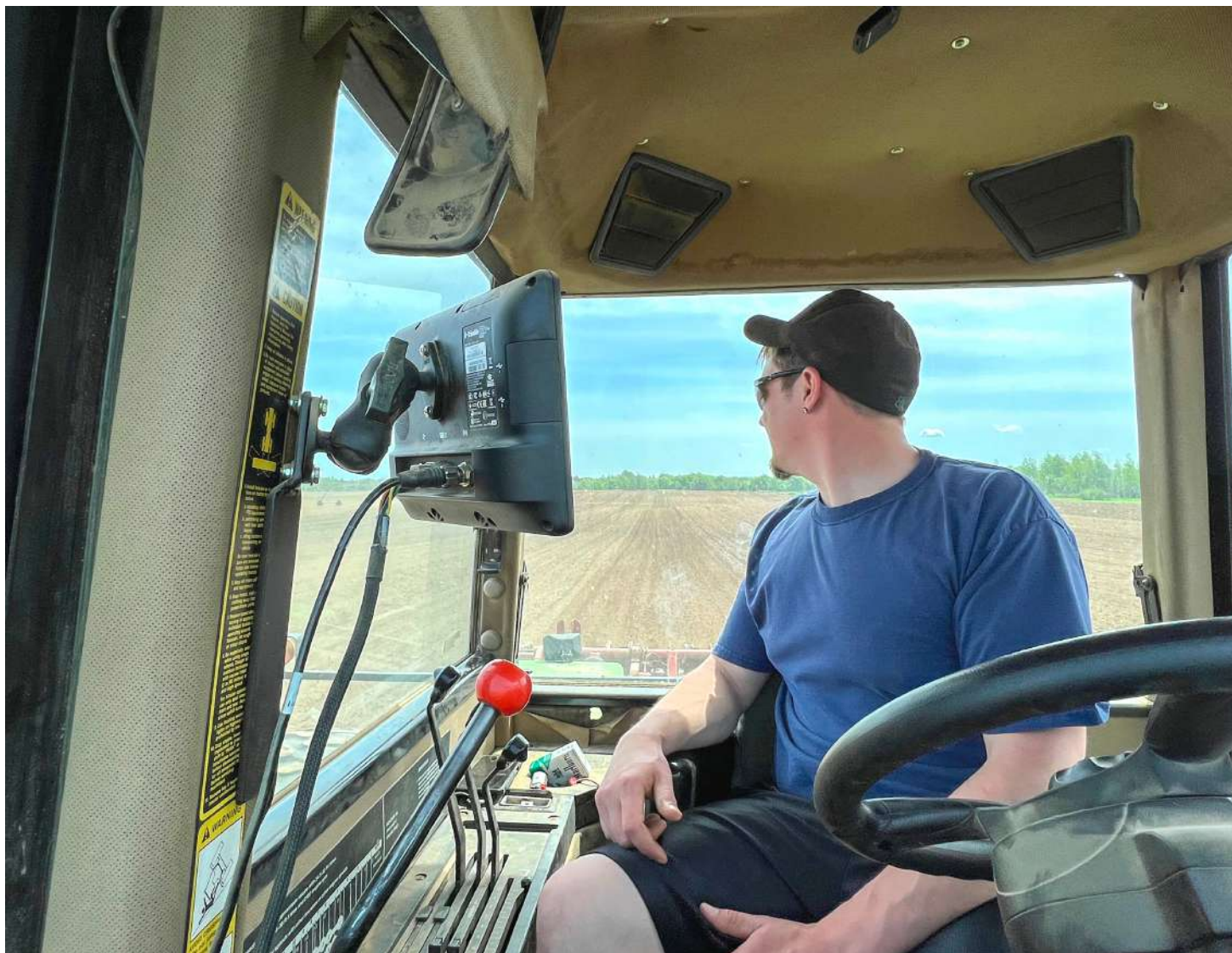
Figure 1: A driver can spend less time worrying if they are driving on their A-B line and more time focused on the work being done with the implement behind the tractor. Driver fatigue becomes less and less of a stress with high accuracy.
