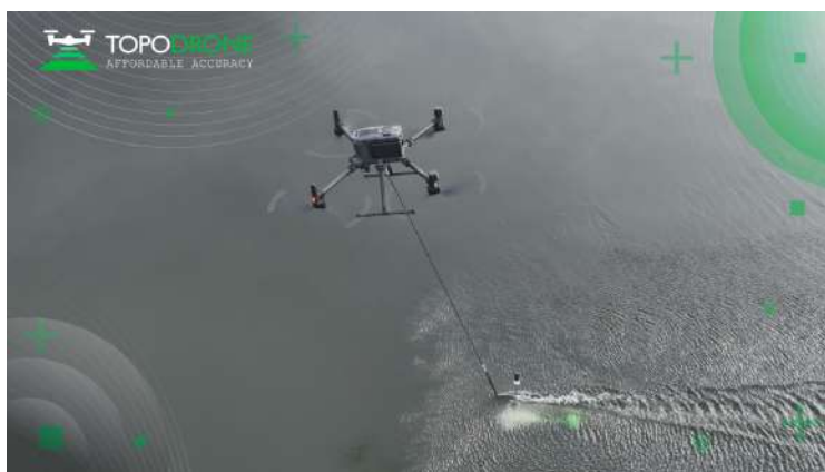
Figure 1: Reservoir surveying with TOPODRONE AQUAMAPPER © TOPODRONE.
