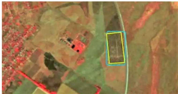
Figure 1: EOS DATA Analytics have developed an algorithm based on remote sensing imagery analysis which constructs a mosaic of the globe every 2 weeks; determining the number of solar plants and calculating their square, average performance, and many other factors.
