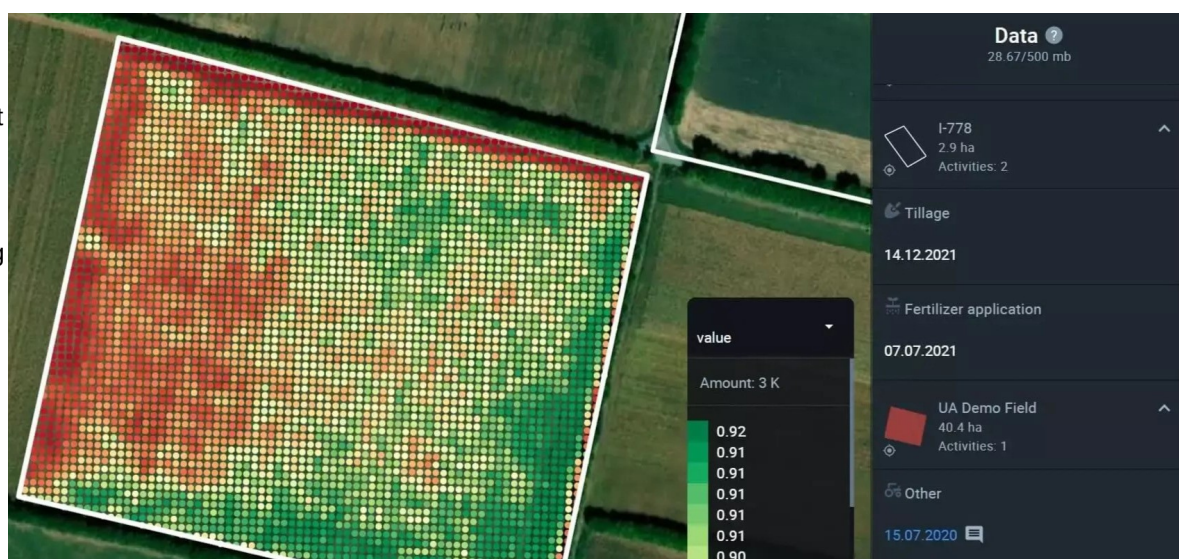
Figure 1: Fertilizer application assessment based on data from field equipment, processed with EOSDA Crop Monitoring.
