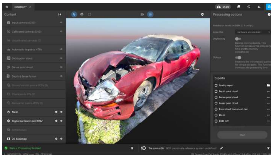
Figure 4: A collision recreated in 3D and processed in PIX4Dmatic.
