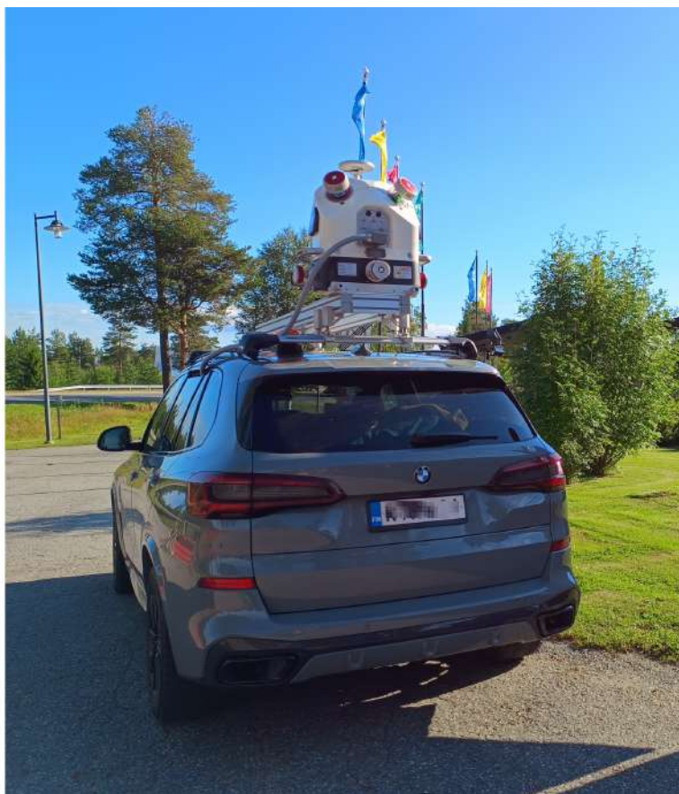
Figure 1: On the left an exploded view of the RIEGL VMX system and on the right the system attached to the surveying vehicle.
