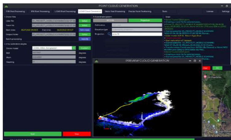
Figure 3: Generation of mobile laser scanning point cloud in real time.
