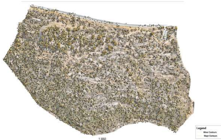
Figure 1: An aerial survey with drones includes contour data, with the lines here marked with black labels.
