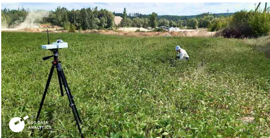
Figure 7: The EOSDA team measures the leaf area index using the SunScan device sensors in the field near Boguslav to confirm EOS SAT-1 satellite measurements. Image: EOS Data Analytics.
