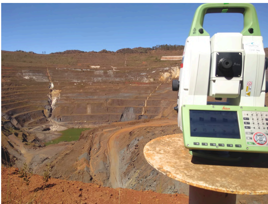
Figure 1: The Leica TM60 facilitates enhanced field workflows and automated data capture processes.
