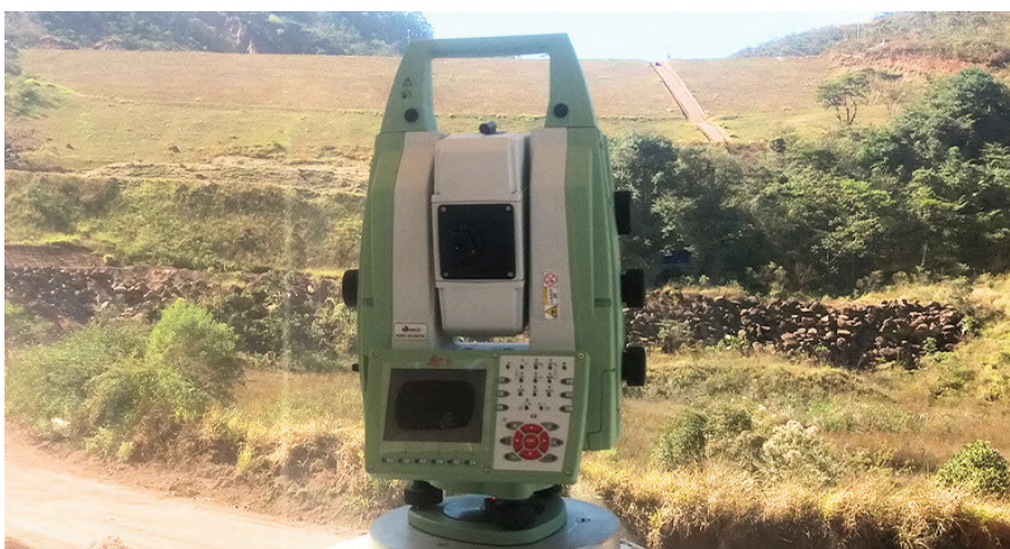
Figure 2: A Leica TM60 is used to observe the precise measurements of the tailing dam embankments.
